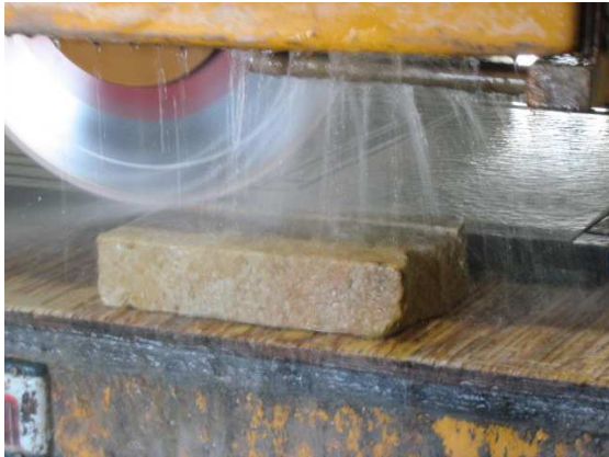
Figure 1: Regeneration of disc in abrasive material
